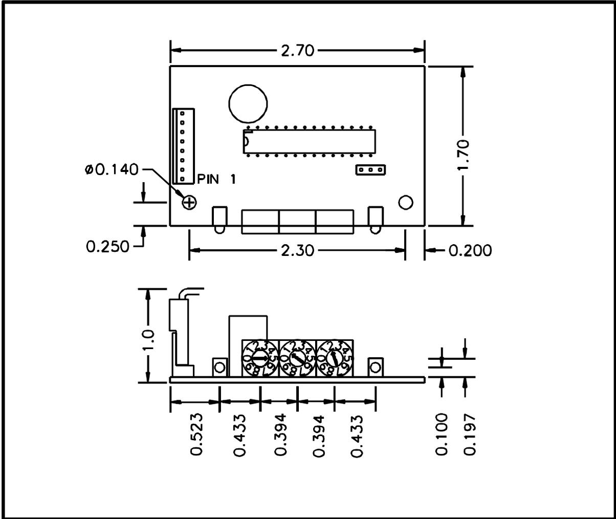
DMX/ONE - Decoder and DMX/ONE - Relay dimensions
