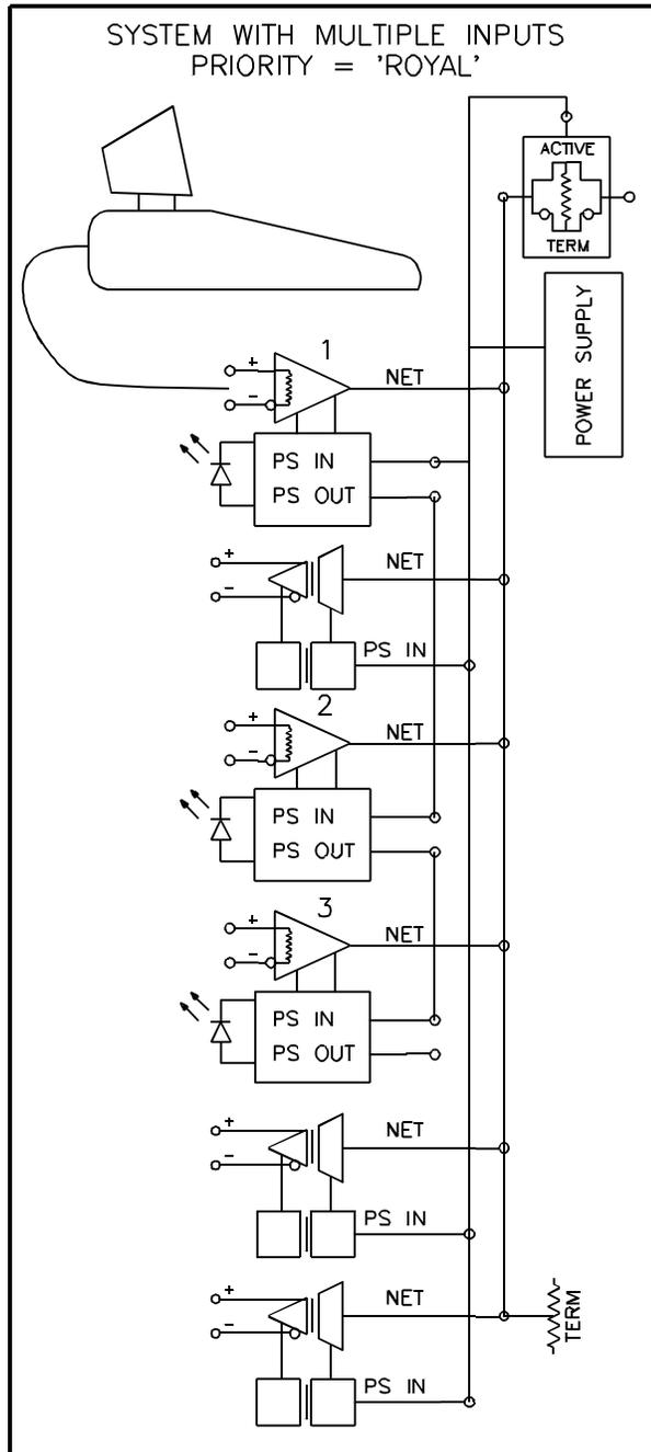
As shown in this layout drawing the input and output modules form a dual terminated EIA485 transmission line. It may be driven at any one point along its length. By buffering the input signal the input modules prevent the cable from the console to input connector from becoming a "Y" in the system. The prioritized switching assures that only one device drives the DMX network.
